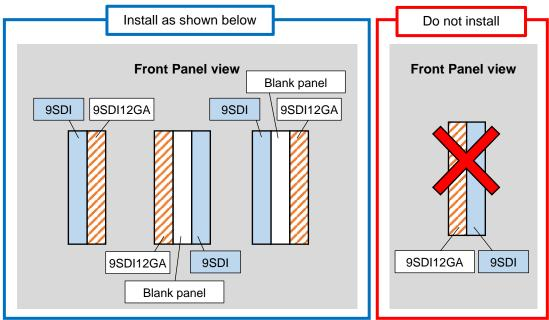
♦ When installing into bottom slots (INPUT 9 to 16 (No. 17 to 20, 29 to 32))
