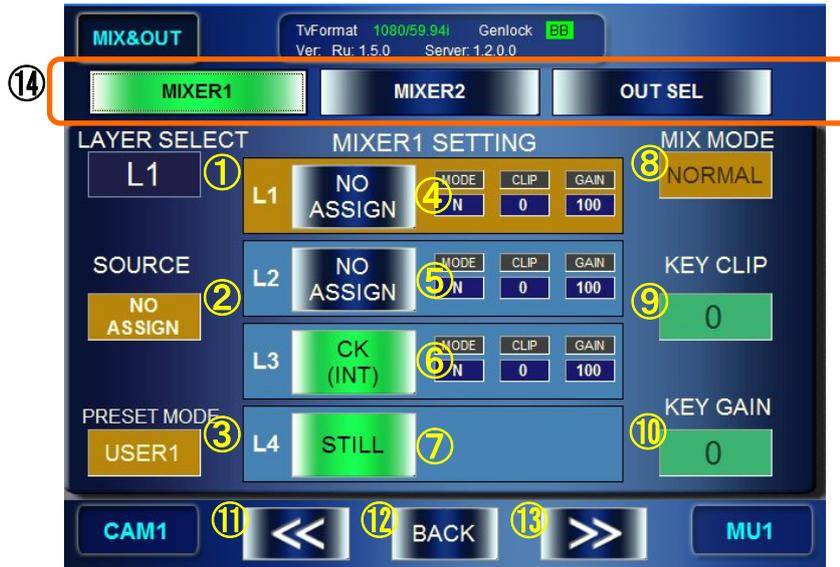
① Select a layer to set Mix Mode, Key Clip, and Key Gain for.
