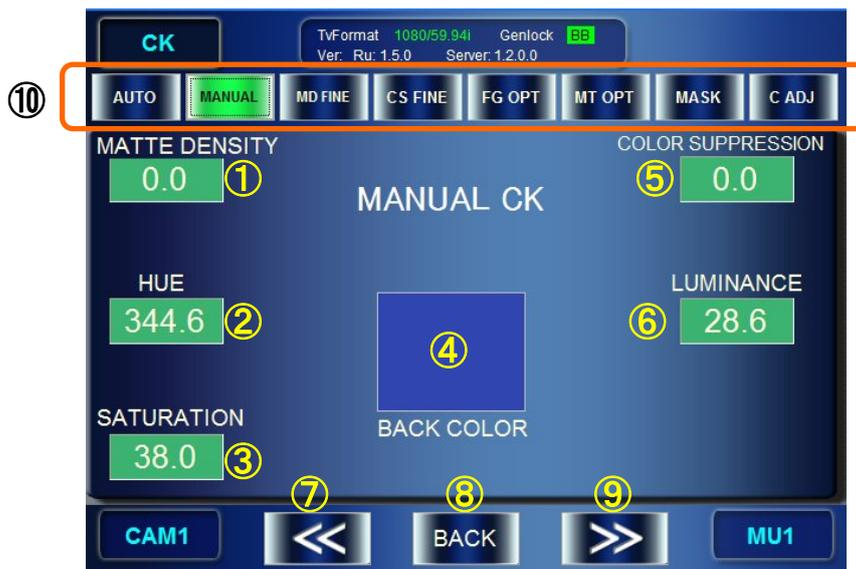
① Adjust the Matte Density (adjust density of matte signal for the backing color with the range of similarity.)
