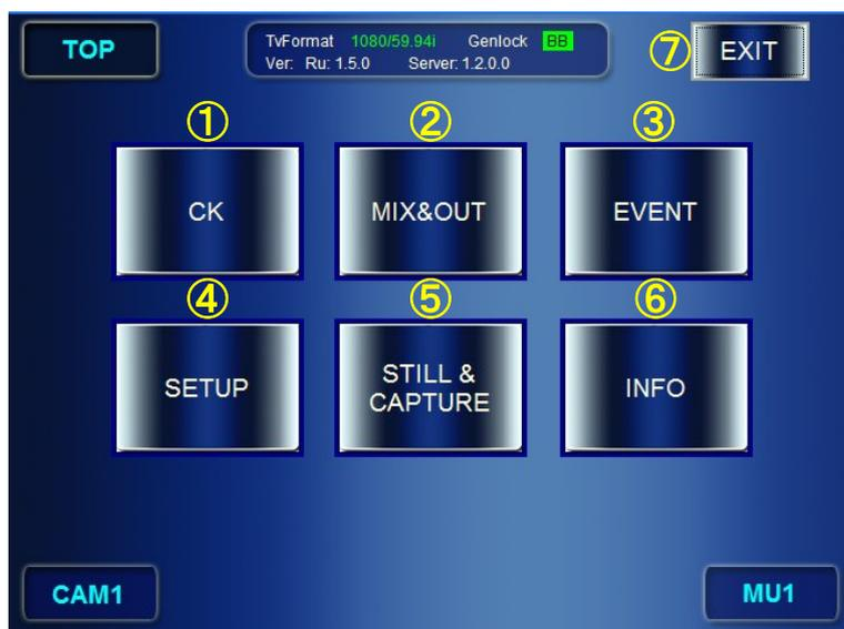
This Top menu is opened by pressing the TOP button on the front panel. The menu buttons provided at the center of the screen allow you to access corresponding menus.
