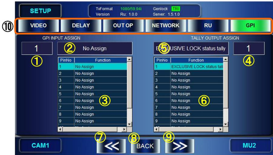
The current input pin assignments are displayed in ③.
