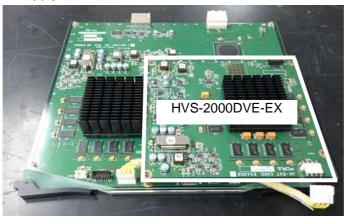
(7) Apply the supplied W sems screws onto the four corners of the HVS-2000DVE-EX card. Connect the power supply cable to the connector.
