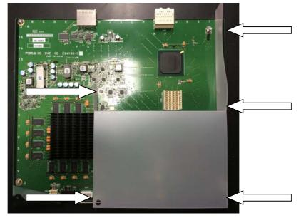
(4) Put the released screws back into the HVS-2000DVE card as shown in the following figure. If the screws to fix the duct in (3) are not stud screws, use the supplied stud screws.
