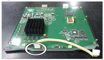
(6) Install the HVS-2000DVE-EX card on the HVS-2000DVE card. Install the HVS-2000DVE-EX card over the power supply cable.
