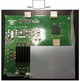
(3) Release the five screws on the HVS-2000DVE card and remove the duct. Keep the removed duct in a safe place.
