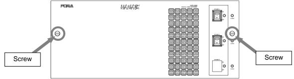
(2) Pull out the HVS-2000DVE card from the bottom slot.
