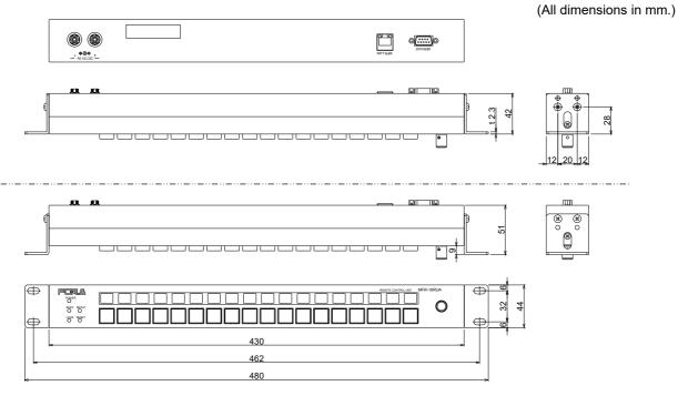
\* The panel buttons can be fitted within the rack by sliding the rack ears forward to attach as shown in the bottom figure above.
