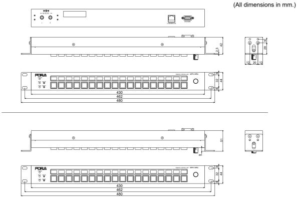
\* The panel buttons can be fitted within the rack by sliding the rack ears forward to attach as shown in the bottom figure above.
