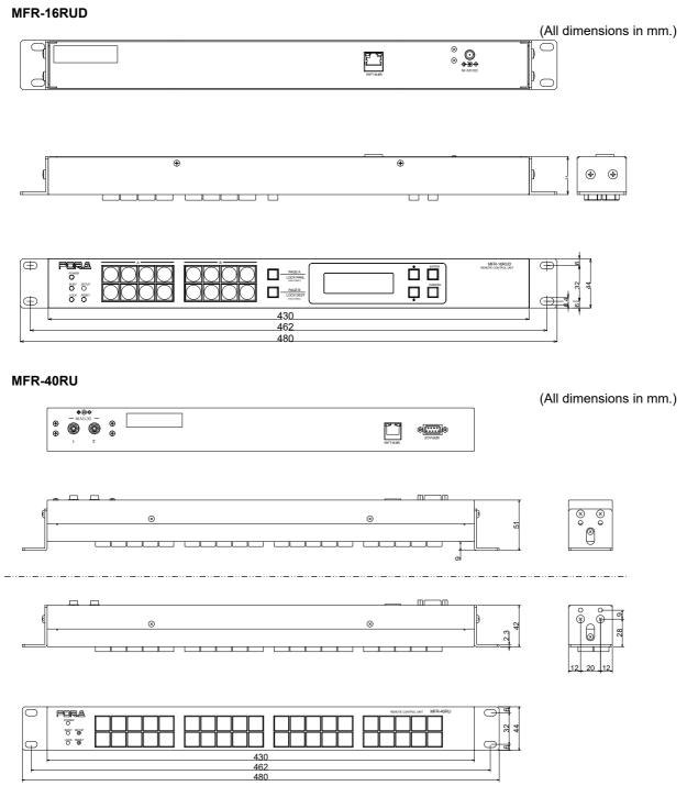
\* The panel buttons can be fitted within the rack by sliding the rack ears forward to attach as shown in the bottom figure above.
