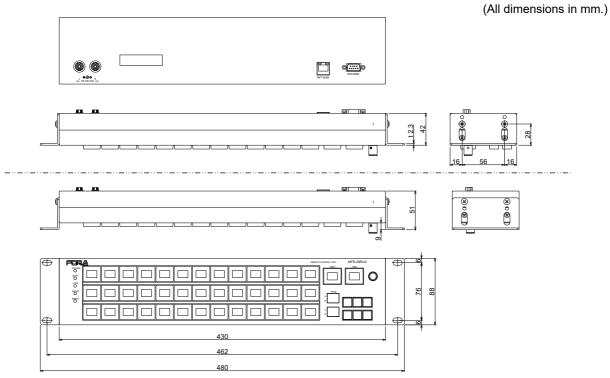
\* The panel buttons can be fitted within the rack by sliding the rack ears forward to attach as shown in the bottom figure above.
