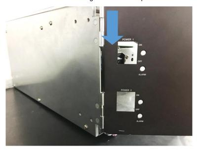
4. Connect the MFR-30FP cable to the connector inside the MFR-3000 as shown below, keeping the red cable edge on top.
