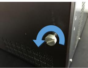
2. Open slightly and slide upward to remove the front panel. If rack mount brackets are applied to MFR-3000, release the rack mount brackets screws.
