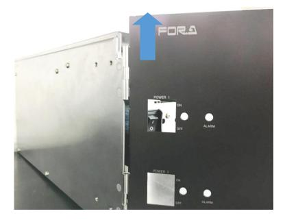
3. Fit the MFR-30FP in hinges and slide the panel down.
