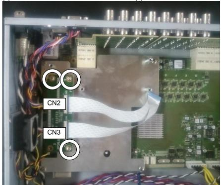
(5) Follow steps (a) to (d) below to connect flexible flat cables to CN2 and CN3 on the IF card.
