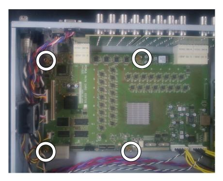
(2) Mount shield plate 1 and secure it with four (4) binding screws.
