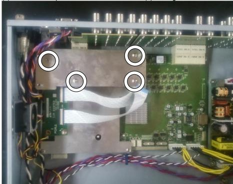
(7) Mount and secure the CPU card with four (4) double SEMS screws.
