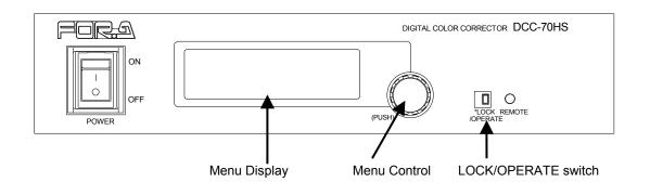
DCC-70HS can disable the front panel menu settings for avoiding the accidental operation. This setting is done using LOCK/OPERATE switch on the front panel.
