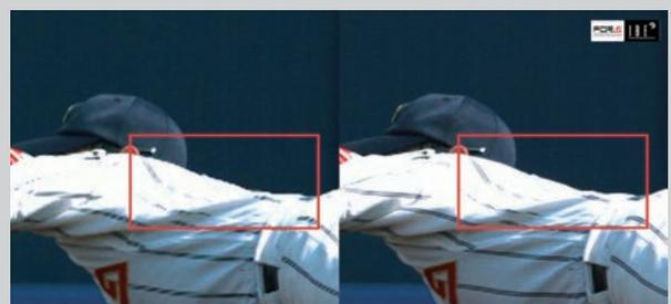
Compared to typical resizing (left), spatiotemporal frame interpolation (right) produces images that are diagonally, significantly smoother.
