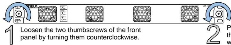
An OPEN alarm sounds intermittently, every 30 seconds, when the front panel is opened. After 5 minutes, the alarm will sound continuously until the front panel is closed. In case the power is on, complete the procedure in a short period of time
