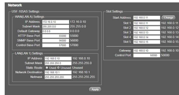
IP addresses are assigned to respective USF-105AS modules installed. Refer to USF-105AS operation manual Sec.10 "USF-105AS Web GUI" for details on setting IP addresses.
