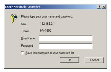
2) Enter the user name and password and click OK. The control screen is displayed when the entered user name and password match the stored data.
