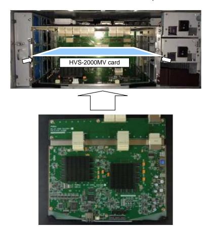
(3) Tighten the two screws at both sides to secure the front panel to the chassis.
