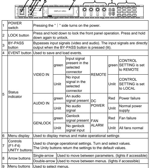
Make sure that the LOCK button LED on the front panel is unlit before starting an operation. If LOCK button LED is lit orange, all operations on the front panel except the LOCK button are disabled. Press and hold the LOCK button to unlock the operations.
