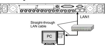
Direct connection using a crossover LAN cable is also possible.
