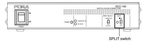
Each time moving the switch up and down changes mode in the sequential order: OFF, 1, 2 and 3.
