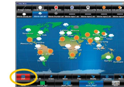
A DSK (composition) function is included. Setting DSK to ON/OFF turns the output on/off for the drawn content (object). With this function, setting to DSK ON enables the drawn content to be output instantly, and when set to DSK OFF, the drawn content is not output until DSK is set to ON. With this button, it is possible to switch at the touch of a button between situations needing real-time drawing and situations needing preparation before output.
