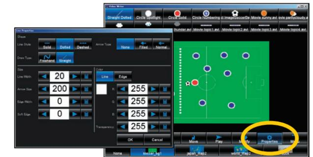
The various buttons assigned to the drawing tools are set by the Properties button. The settings of placed objects are changed with the Modify button.
