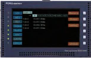
Measures video delay, audio delay, relative delay between audio channels, or relative delay between video and audio, based on test time code signals.
