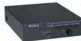
Besides vertical and horizontal camera shake, the IVS-200 corrects rotation camera shake and comes with FOR-A's Auto Video Optimizer (AVO) function that automatically adjusts video levels.
