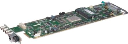
Modular SDI changeover switcher for USF-105AS or USF-212AS/212BS frames (p.18). Monitors status of two SDI inputs and seamlessly switches to the error-free line if errors are detected.
