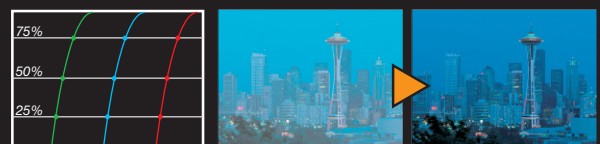
RGB independent gamma adjustment in HIGH (near 75%), MID (near 50%) or LOW (near 25%) tone.
