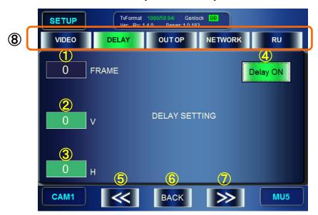
① Display / Set the number of frames of Camera delay Indication: Shows the value of the current setting.
