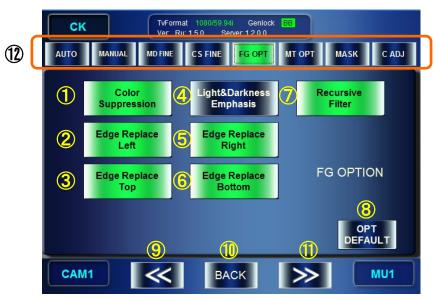
① Turn ON/OFF the filter for vertical direction implemented when generating mattes. Setting ON will smooth the vertical edges of mattes.
