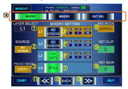
① Select a layer to set Mix Mode, Key Clip, and Key Gain for. Indication: Shows the currently selected layer.
