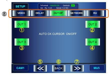
① Set to display or not to display a cursor on the VIDEO OUTPUT1 output image. Indication: Shows the value of the current setting.
