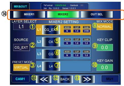
① Select a layer to set Mix Mode, Key Clip, and Key Gain for. Indication: Shows the currently seleced layer.
