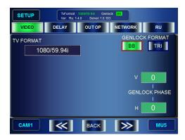
4) Turn the top left knob and select a TV standard, then press the knob to confirm the selection. The massage "Do you want to change video format?" appears. Select **OK**. Then the TV standard will be changed.
