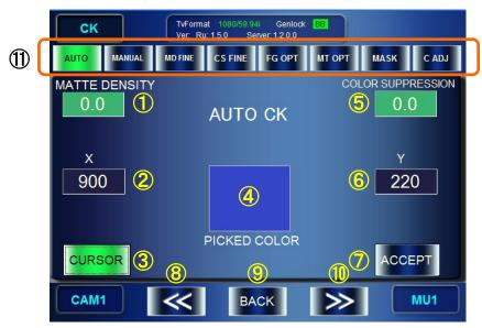
Adjust the Matte Density (adjust density of matte signal for the backing color with the range of similarity.)
