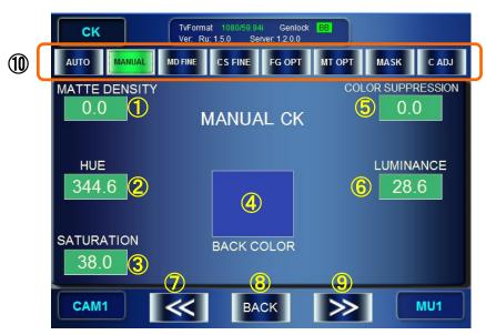
① Adjust the Matte Density (adjust density of matte signal for the backing color with the range of similarity.)
