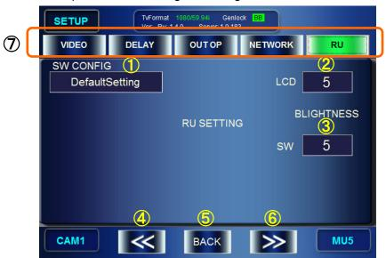
① Open the SW CONFIG(configuration of buttons on the front panel) selection panel
