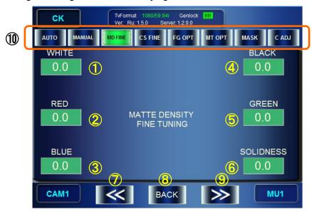
① Adjust the density of matte signal for the backing color which includes white component. For example, if the selected backing color is blue, you can adjust the density of matte signal for whiteish blue backing color.
