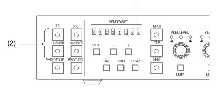
Repeatedly press the button until the desired ID is selected. The selection is changed as below every time the button is pressed.
