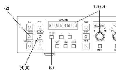
If the destination device is not found, the light on the <u>VIDEO LEVEL</u> control knob blinks and the related button light goes off. In this case, repeat steps (1) to (6), specifying the slot number where the destination device (UFM-30DCC) is installed.
