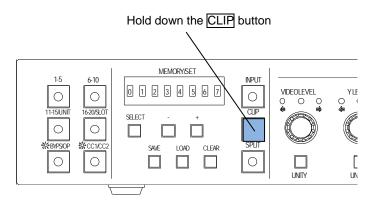
(3) Once the setting is complete, press the CLIP button to return to Color Correction mode.
