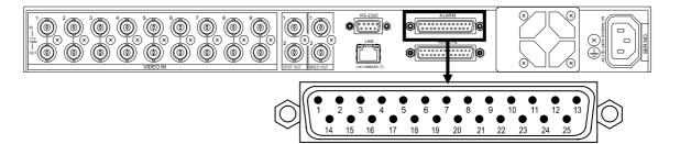
• Connector Pin Assignment Table (25-pin D-sub male)
