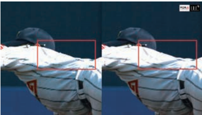
Compared to typical resizing (left), spatiotemporal frame interpolation (right) produces images that are diagonally, significantly smoother.
